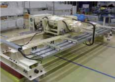
Clean Room Crane(2Ton)
